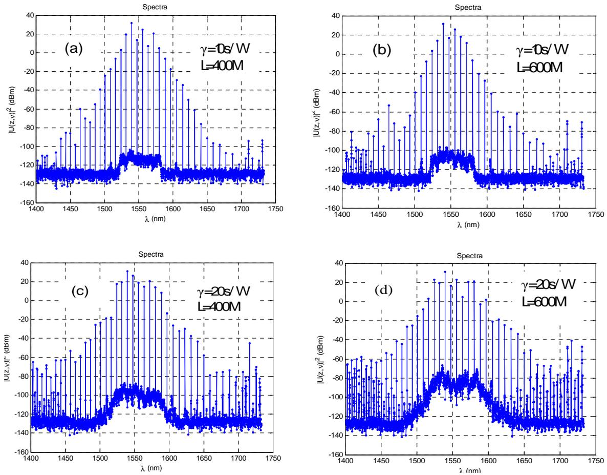
Fig.2: Power variation against wavelength at a)  $\gamma=10$  s/W,  $L= 400$  m, b)  $\gamma=10$  s/W,  $L=400$  m, c)  $\gamma=20$  s/W  $L=400$  m and d)  $\gamma=20$  s/W,  $L=600$  m.
