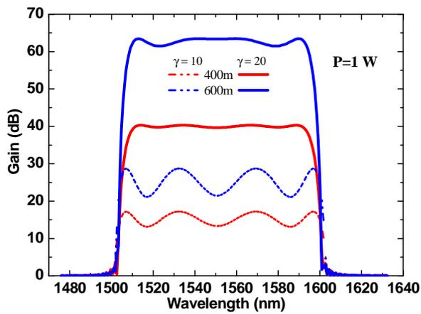
Fig.3: Graph of gain against wavelength at different values of  $\gamma$  for 400 m and 600 m fibre lengths.
