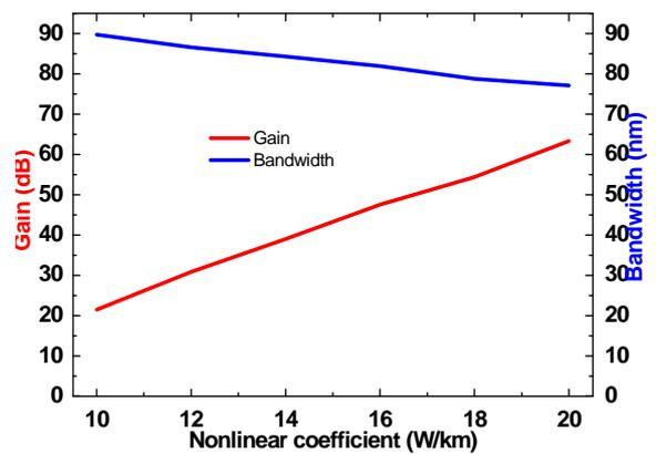
Fig.4: Graph summarizing the relation between Gain, Bandwidth and Nonlinear coefficient.
