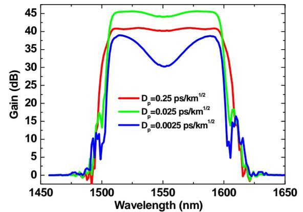
Fig.8: Graph of gain at different Polarization Mode Dispersion (PMD) coefficients,  $D_p$ .
