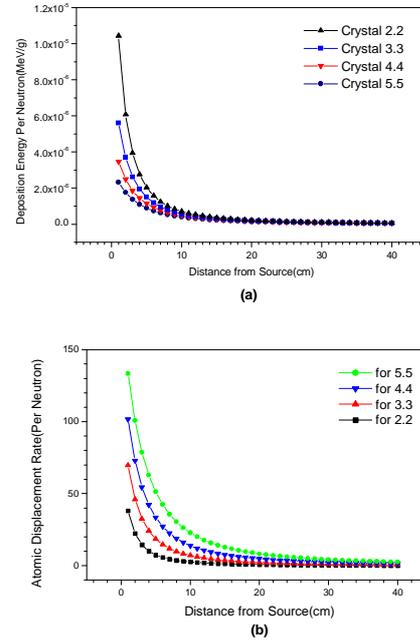
Fig. 1: (a) Energy deposition per gram in different Ge crystal due to an Am-Be source; (b) the atom displacements rate.
