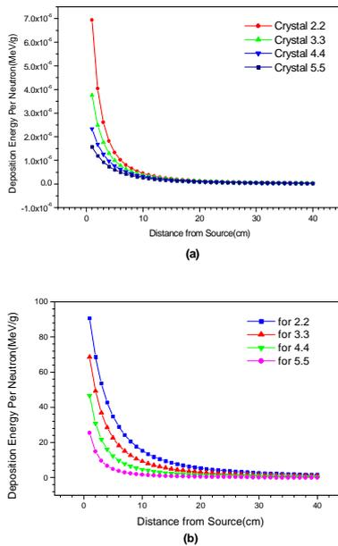
Fig. 3: (a) Energy deposition per gram in different Ge crystal due to a  $^{252}\text{Cf}$  source; (b) the atom displacements rate.
