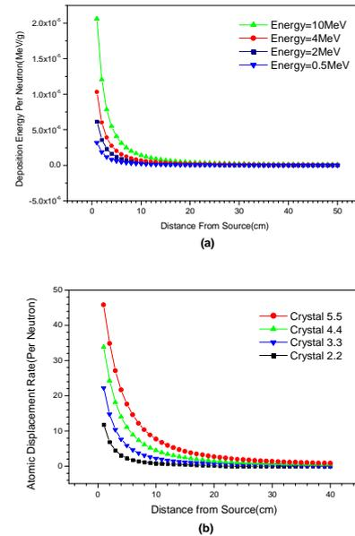
Fig. 2: (a) Energy deposition per gram in 2"×2" Ge crystal due to different mono-energy point sources; (b) the atom displacements rate.
