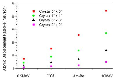
Fig. 4: Comparison of atom displacements rate in Ge crystals that placed on 10 cm of different sources.
