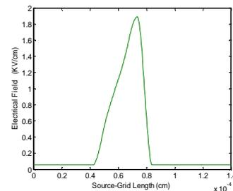
Fig.1: Electrical field variation in the channel.
