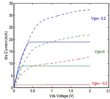
Fig.7: Experimental-theoretical comparison for  $I_{ds}(V_{ds}, V_{gs})$  characteristics.
