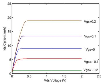
Fig.4:  $I_{ds}(V_{ds}, V_{gs})$  characteristics.
