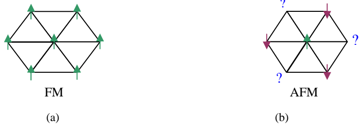
Fig.5: a) Hexagonal lattice with no frustrated spins in FM interaction. b) Hexagonal lattice with frustrated spins in AFM interaction: the so-called geometric frustration. As one can observe in this second case, there is no spin configuration and where all the spins have their lowest interaction energy. As a result, there is no clear ground state configuration.
